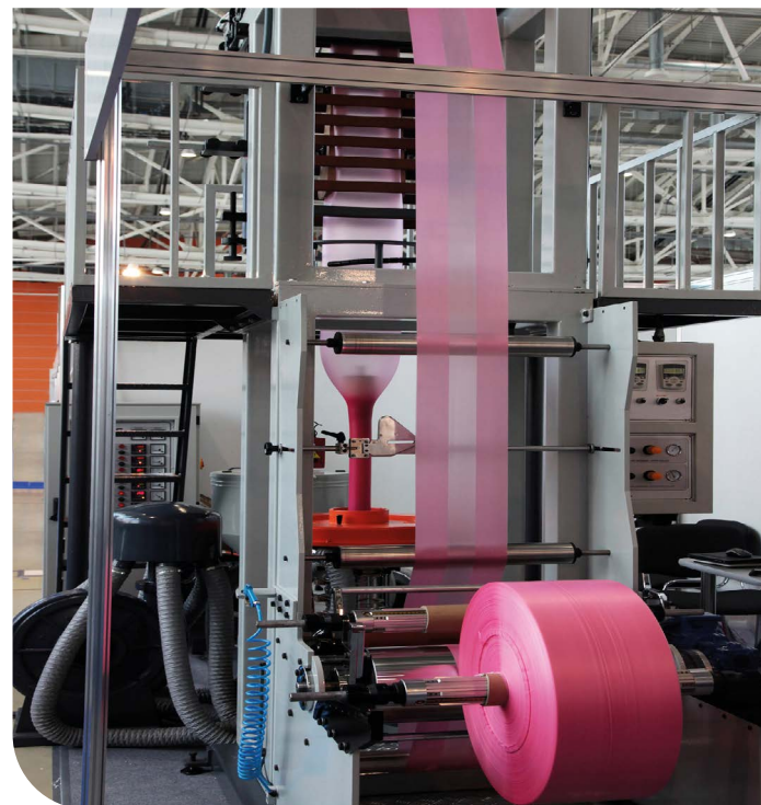
Temperature-proof hoses used for extracting hot air for the manufacturing of bubble packaging
