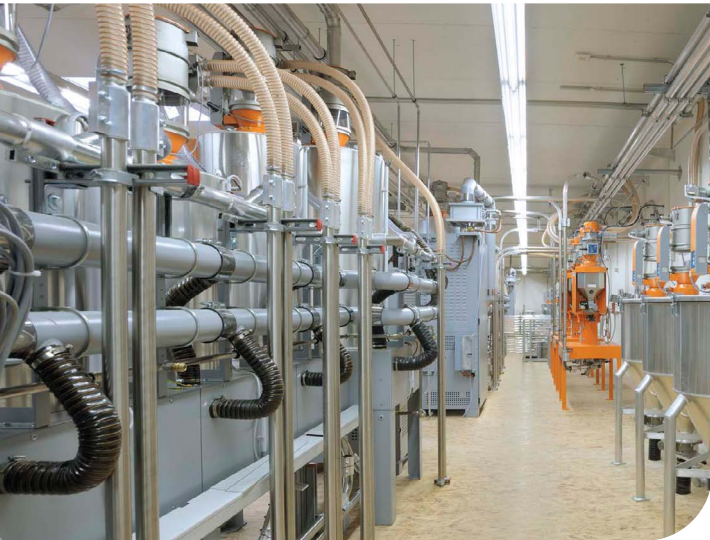
Suction & transport hoses used for filling granule dryers along with temperature-proof hoses for transporting the air for the dryer itself
